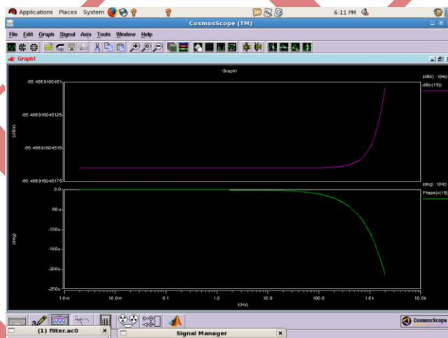
Fig.6 Frequency response with the cutoff frequency 300Hz and phase
