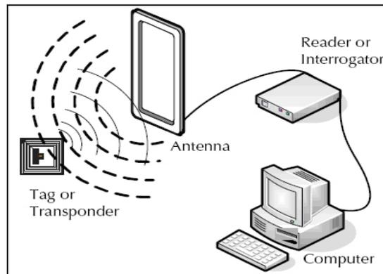
The RFID system has three components, these are:
