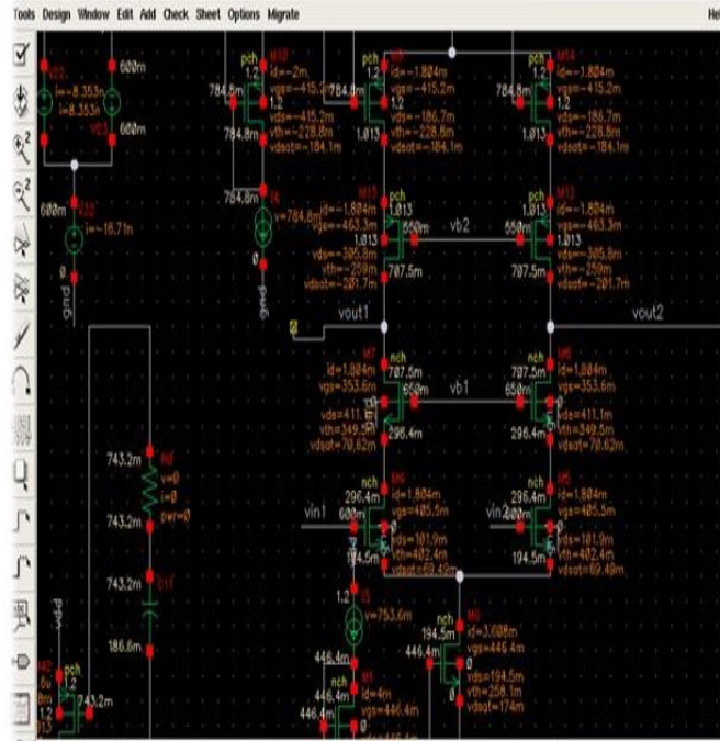
Fig 15. Sample and Hold Circuit in Cadence
