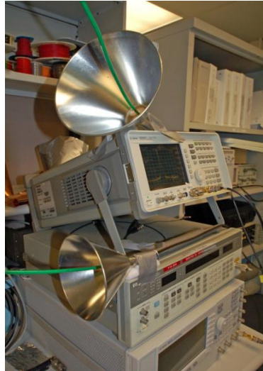
Figure 5 : Two-ended Cable Test Setup Utilizing the Test Points to Launch and Receive the RF Probing Signals
