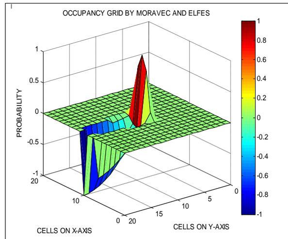
Fig.3 3D View of Occupancy Grid Modeling for Ultrasonic Range Finder
