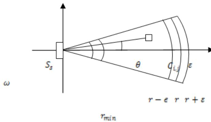
Fig.2 Field of View of the Sonar Sensor
