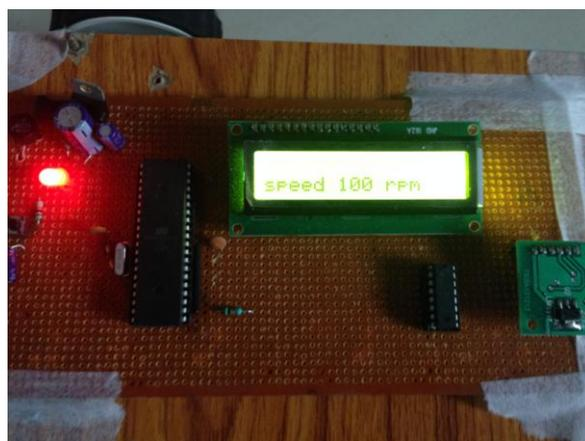
**Fig. 6** When the vehicle is moving on a flat road, the motor is running at a speed of 100 rpm.
