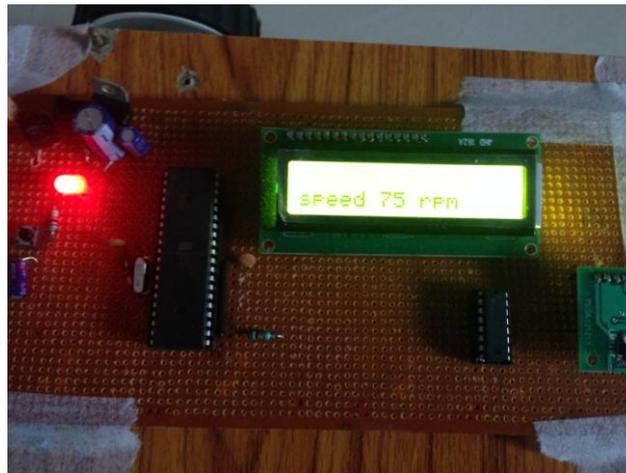
**Fig. 7** When the vehicle is moving on a road with a elevation of 100, speed restricted to 75 rpm
