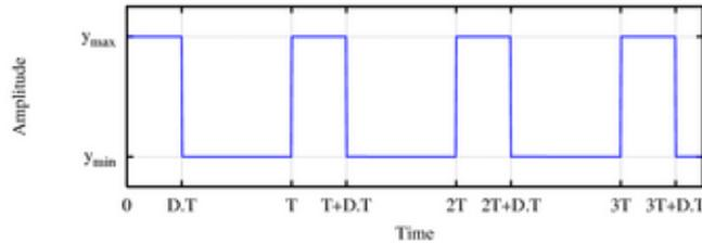
**Fig. 3 Square Wave, Showing the Definitions of  $y_{min}$ ,  $y_{max}$  and Duty Cycle**
