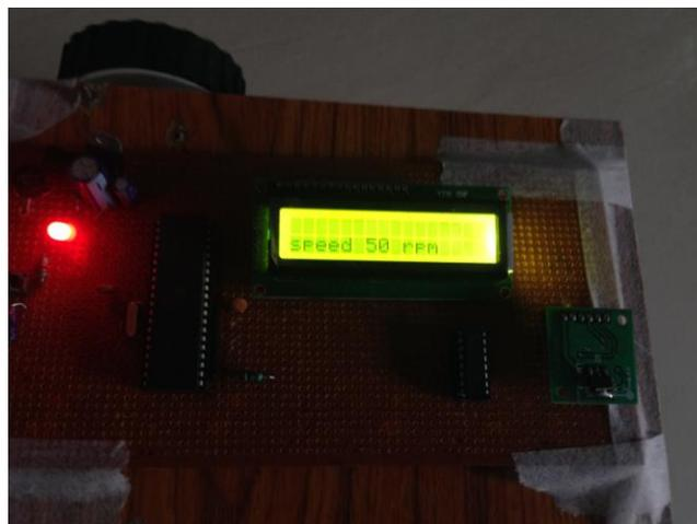
**Fig 8.** When the vehicle is moving on a road with a elevation of 200, speed is limited to 50 rpm
