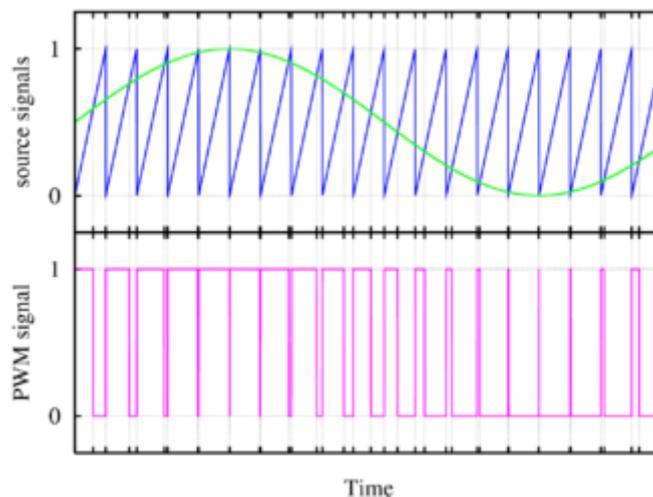
**Fig. 4 Pulse Width Modulation Signal Graph**
