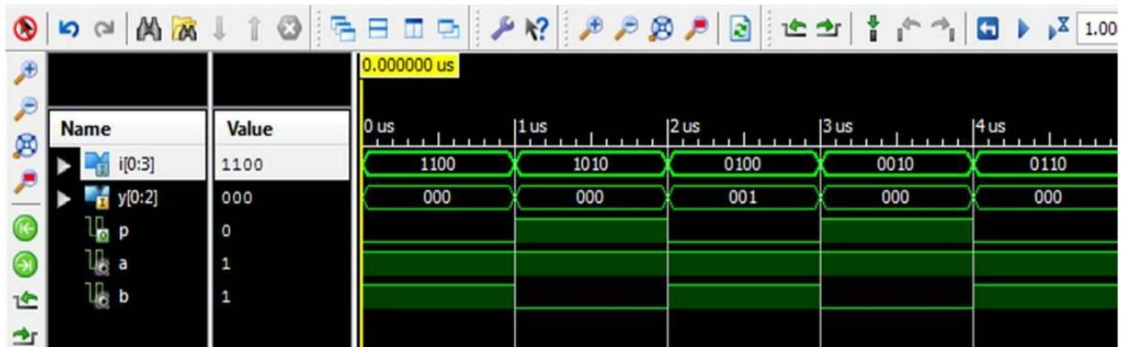
**Figure5. Detection of slow to fall (1→0) fault at line 14 of s27 circuit by skewed load test**
