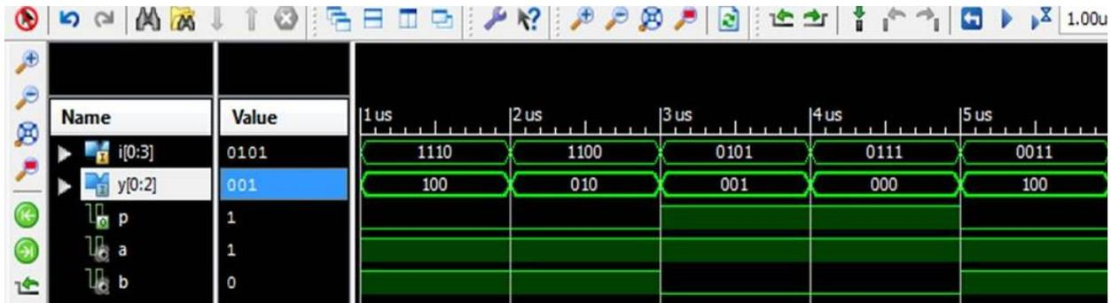
**Figure4. Detection of slow to fall (1→0) fault at line 9 of s27 circuit by skewed load test**
