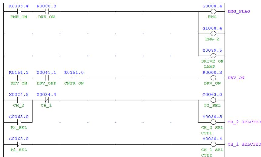
**Figure 3: Introductory Ladder programming**
