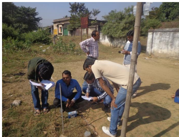
Fig.3. monitoring of ground vibration with minimate
