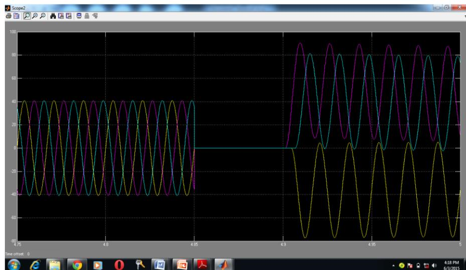
**Fig 5. Output voltage with 3 phase fault**
