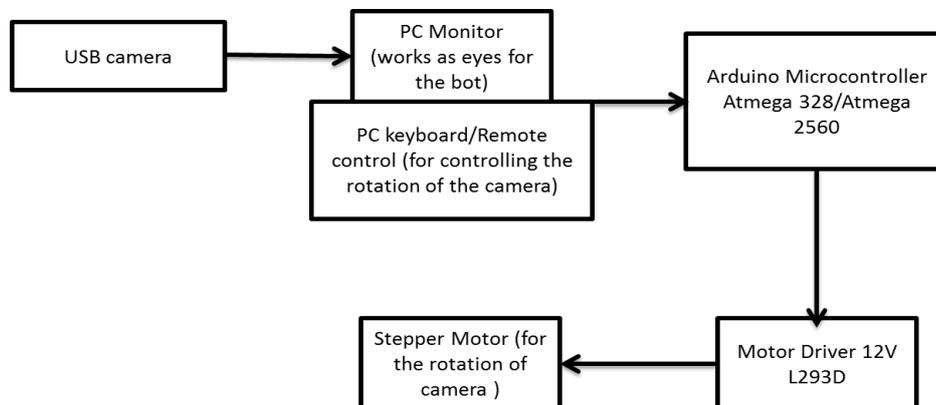
**Fig.2: Block Diagram for Rotation of Camera**
