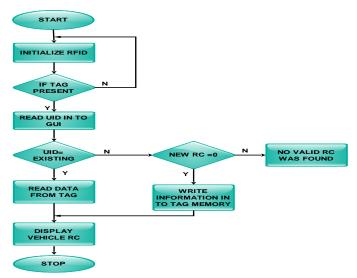
Figure 3: Flowchart for Vehicle Registration And Identification System.
