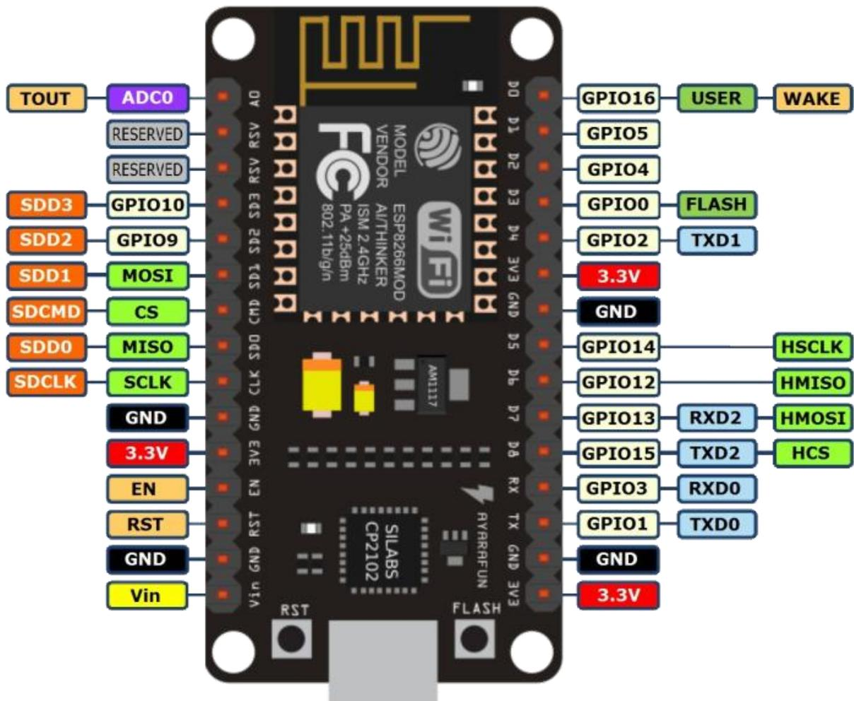
Node MCU is an open-source IOT platform. It includes firmware which runs on the ESP8266 Wi-Fi SOC from expressive systems and hardware which is based on the ESP-12 module. The term NodeMCU by default refers to
