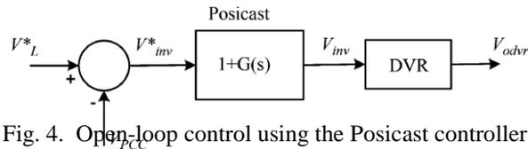
Fig. 4. Open-loop control using the Posicast controller.
