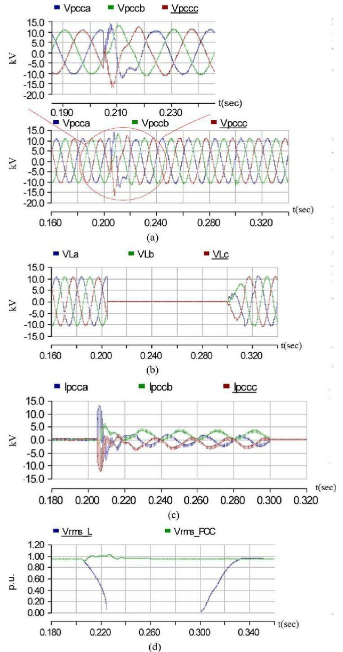
Fig. 12. Fault current limiting by DVR.
