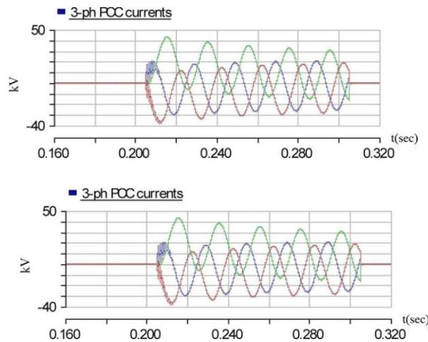
Fig. 13. Current wave shape due to the three-phase short-circuit fault without DVR compensation.
