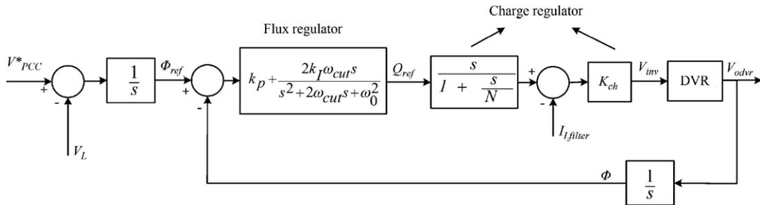
It should also be noted that the reference flux ( $\Phi_{ref}$ ) is derived by integration of the subtraction of the PCC reference voltage ( $V^*$ ) and the DVR load-side voltage. In this control strategy, the control variable used for the outer flux model is the inverter-filtered terminal flux defined as:
