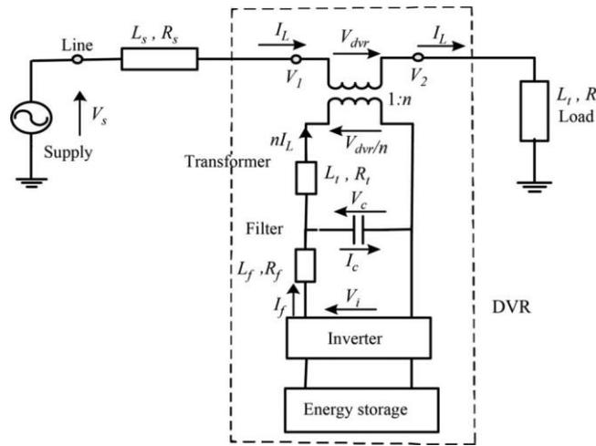
Fig. 3. Distribution system with the DVR.
