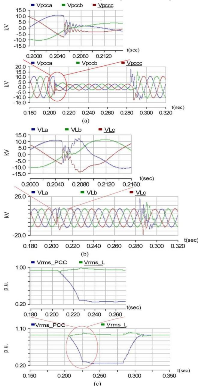
Fig. 10. Three-phase fault compensation by DVR. (a) Three-phase PCC volt-ages. (b) Three-phase load voltages. (c) RMS voltages of PCC and load.
