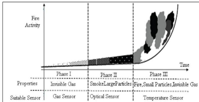
Fig.5 Fire Characteristics diagram
