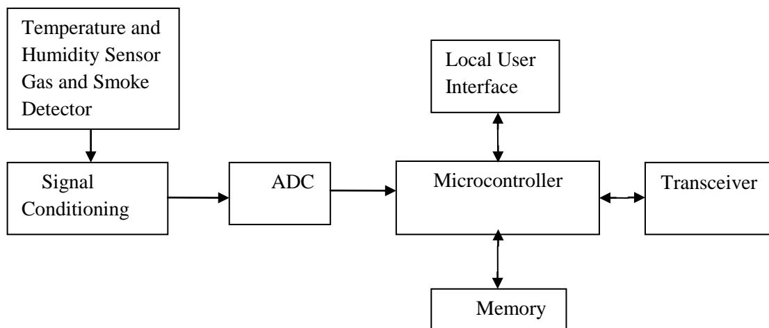
Fig.3 Components of a Sensor node
