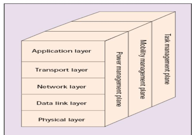
Fig 2. Wireless Sensor Network Protocol Stack
