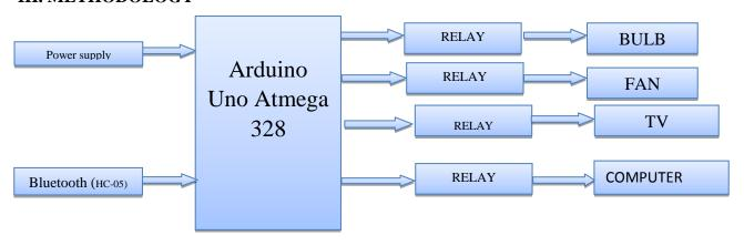
Fig3: Shows block diagram of voice control based home appliances using android devices on Arduino In this block diagram we have two sections are there. Firstly Bluetooth is communicating with at mega 328 microcontroller.
