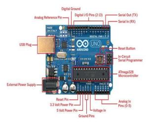
Fig2 shows Arduino Uno board with electrical input output pins
