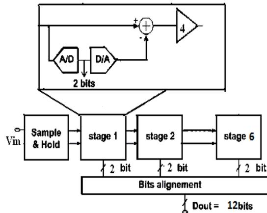
**Figure 2** Block diagram of proposed pipeline ADC
