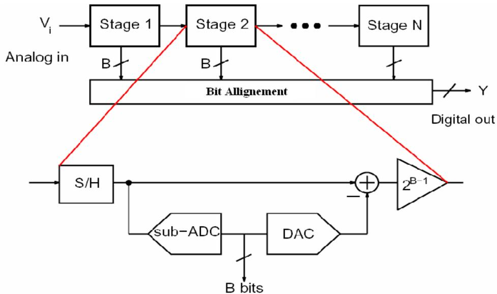
**Figure.1 Block diagram of a pipelined ADC**
