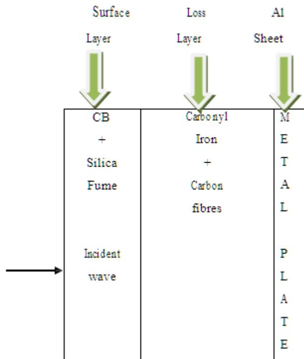
**Figure. 5: Structure of Proposed Cement-based Radar Absorbent**
