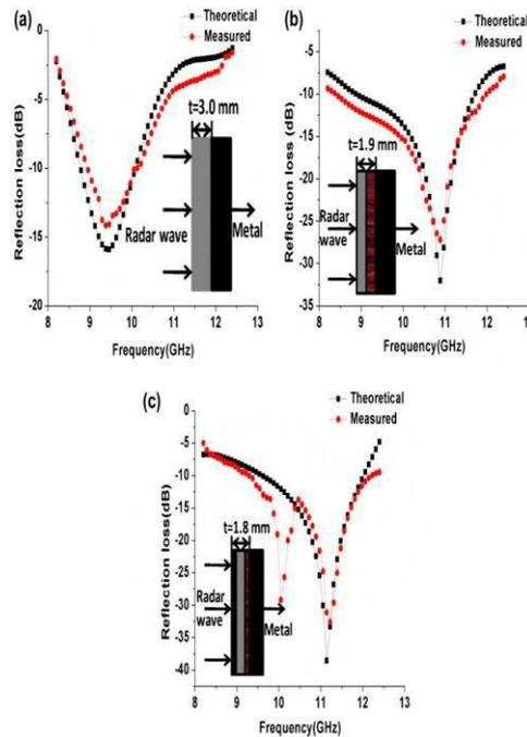
**Figure 4. Measured RL of (a) single layer of M1 with thickness 3.0 mm
