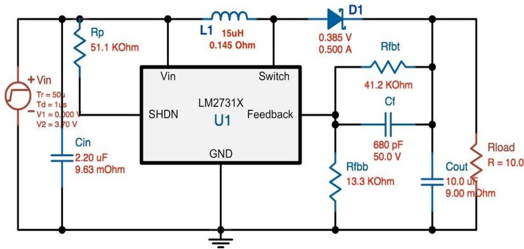
Fig 4.1 LM2731 boost converter
