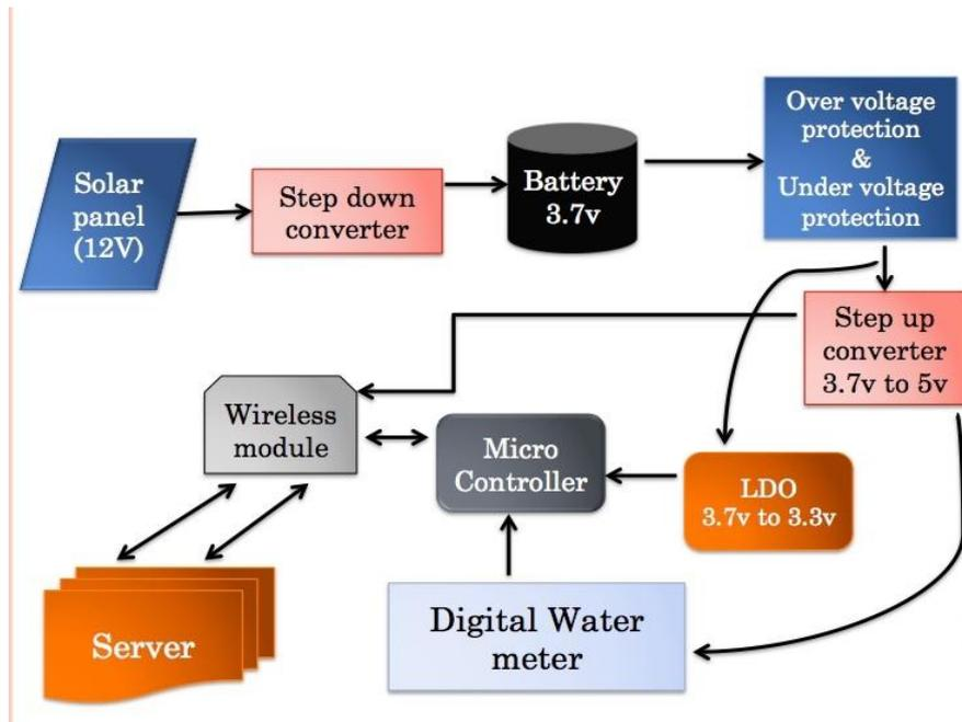
**Fig 2.1 Block diagram**
