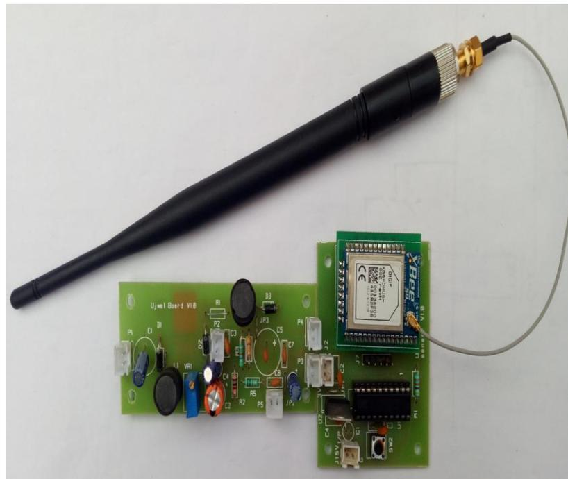
**Fig 7.2 Hardware of converters, microcontroller and ZigBee**
