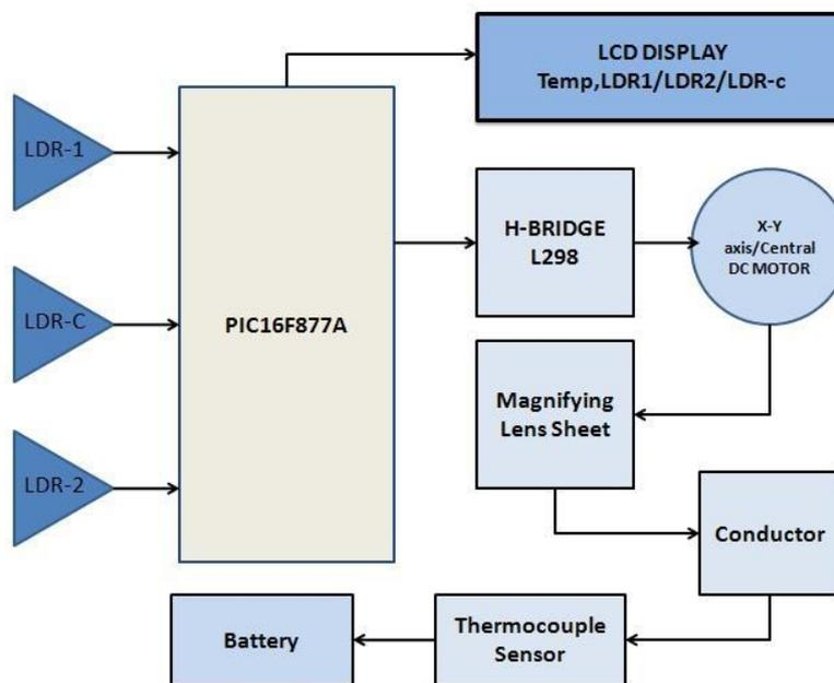
**Figure 2. Hardware Implementation of Solar Tracking system**
