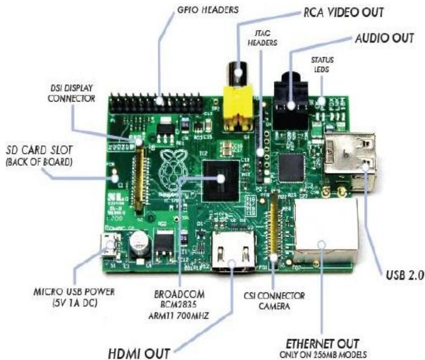
**Fig.2 Raspberry Pi Microcontroller Board**
