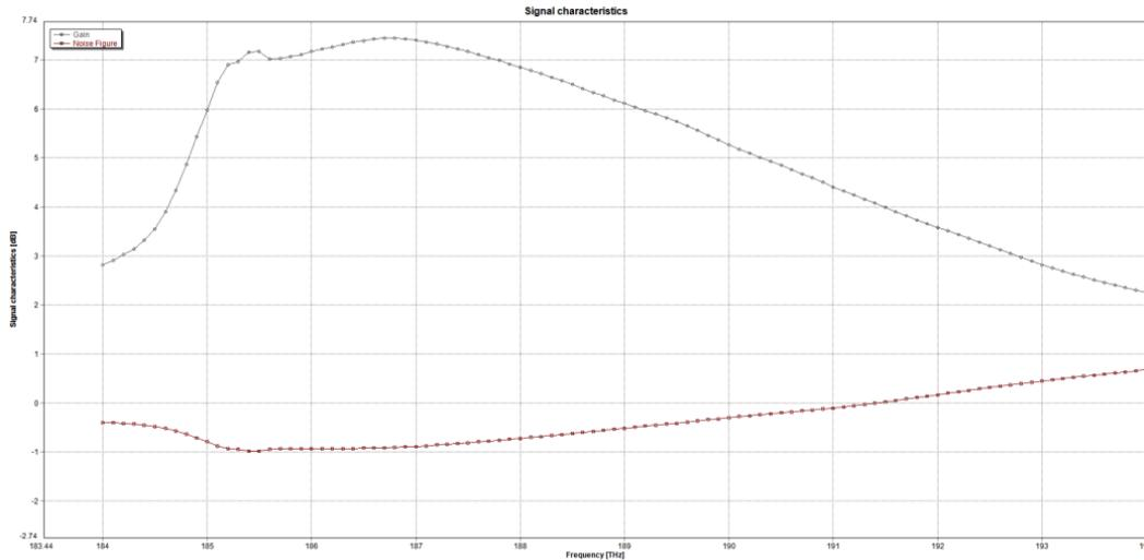
**Figure 3: Gain and NF of Raman amplifier when co-counter pumped with 1500 nm and 1502 nm respectively**
