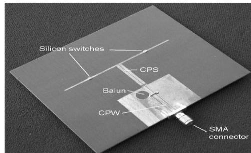
**Fig. 5. Photograph of the switched dipole antenna [9]**
