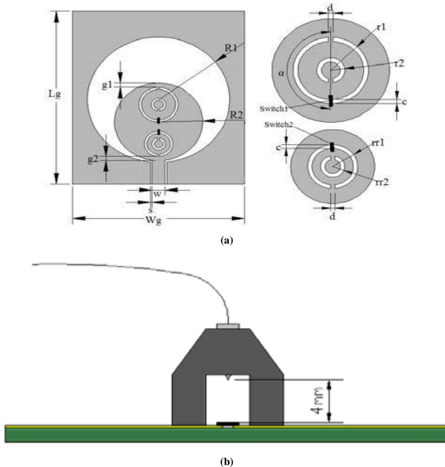
**Fig 2 (a) proposed antenna; (b) fiber installation for the optical control of the proposed antenna [3]**
