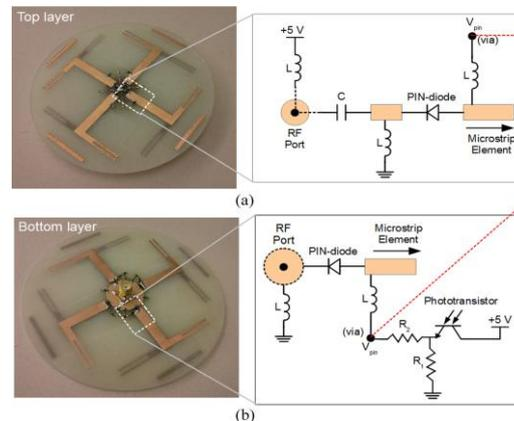
**Fig. 6 optical switching circuitry for a pair of symmetric elements. (a) Top biasing circuitry. (b) Bottom optical and biasing circuitry. The voltage and current activated by the phototransistor.**
