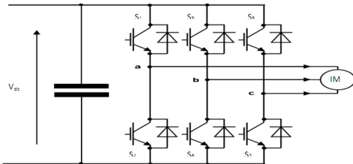
**Fig 1. Three phase VSI using MOSFETs**
