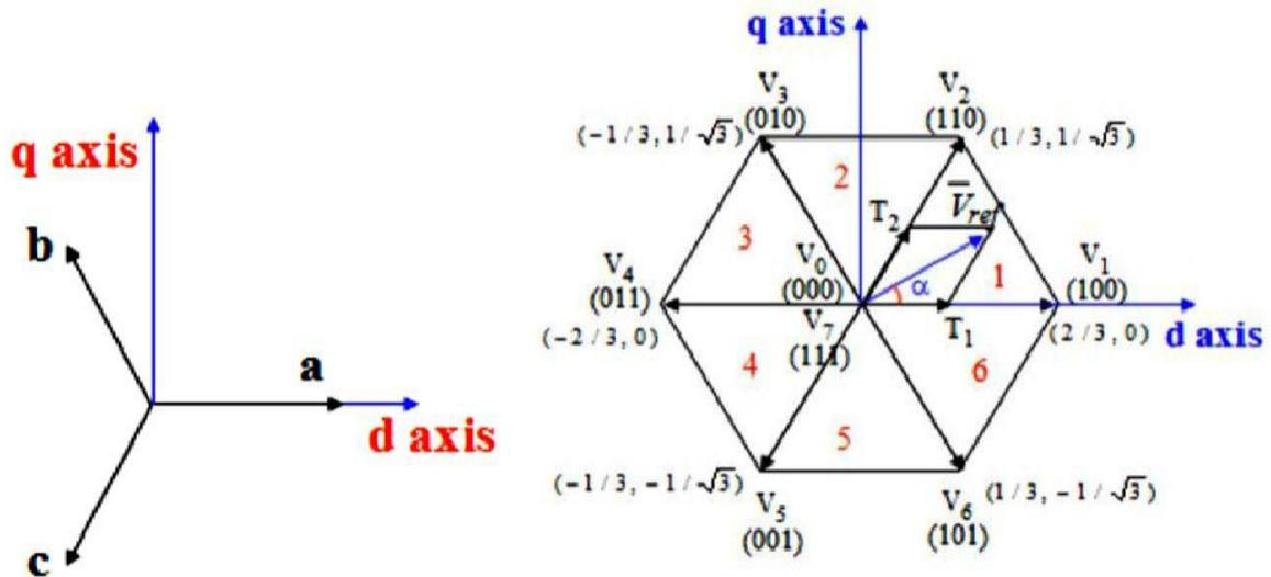
**Fig. 2. abc-dq transformation and space vector trajectory.**
