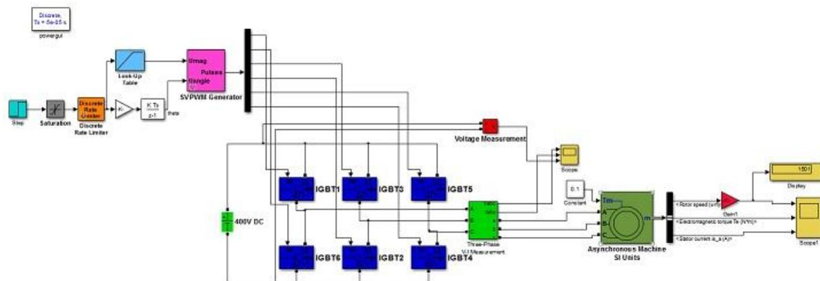
**Fig. 3 MATLAB Simulation SVPWM Inverter**
