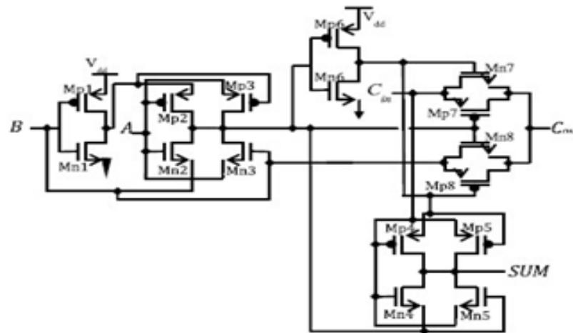
**Fig.2. Hybrid CMOS Full Adder**
