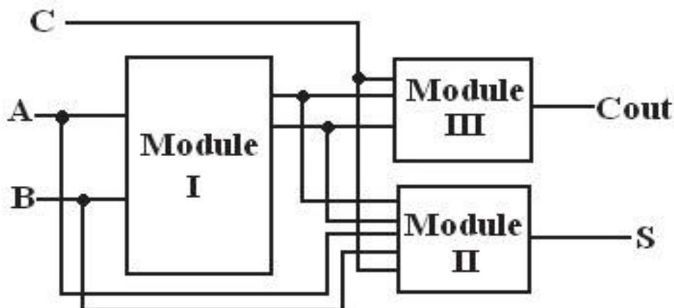
**Fig.1. Full Adder Logic Architecture with Three Modules.**
