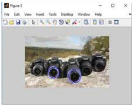
Fig. 5 cameras having radius (pixel difference) in range between 15-30
