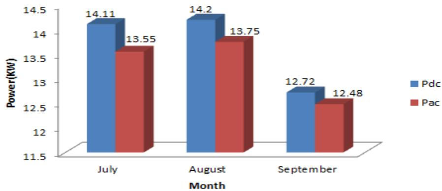
**Fig.13.Average DC power output and converted AC power for three months**
