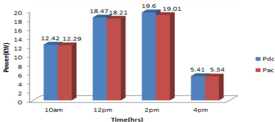
**Fig.10.DC power output and converted AC power Per Day**
