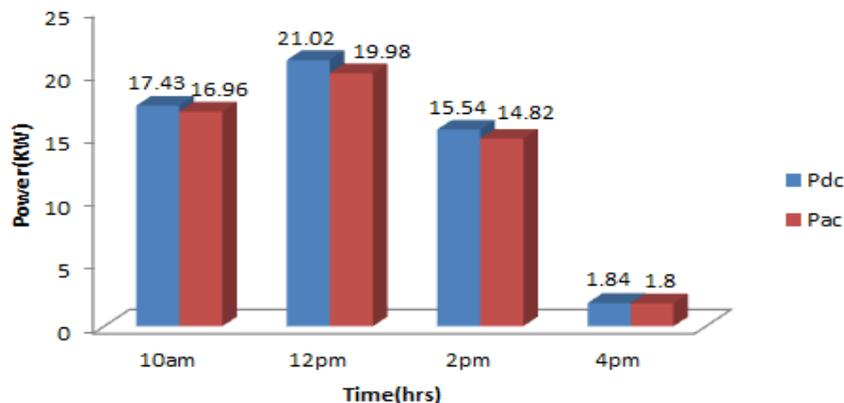
**Fig.4.DC power output and converted AC power Per Day**
