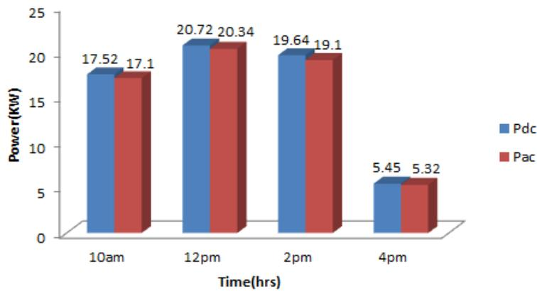
**Fig.7.DC power output and converted AC power Per Day**
