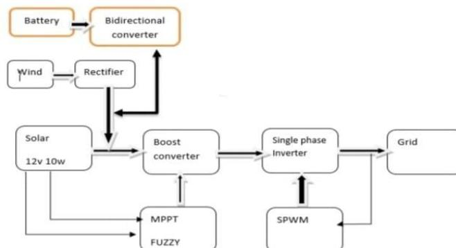
**Fig.1 Studied Block Diagram of MG System**
