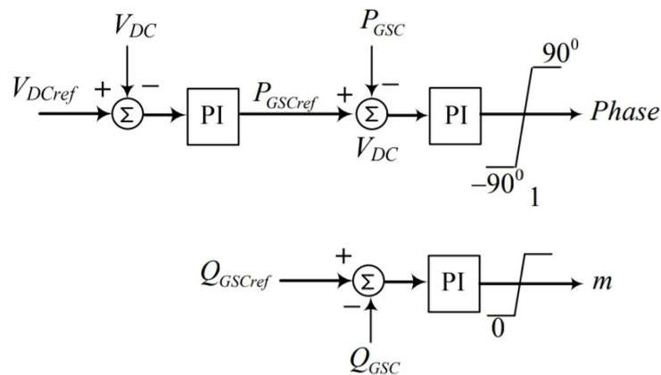
**Fig 3. Control Scheme Of GS**
