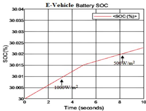
**Fig 4.3.3 Change in SOC (%) vs. time 1000W/m2**
