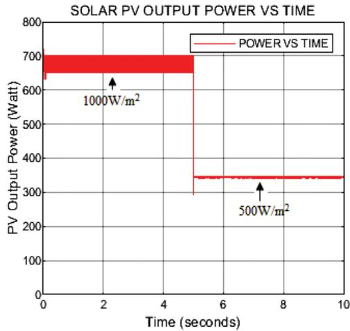
**Fig 4.3.1 PV output Power vs. Time at 1000W/m2 and at 500W/m2**
