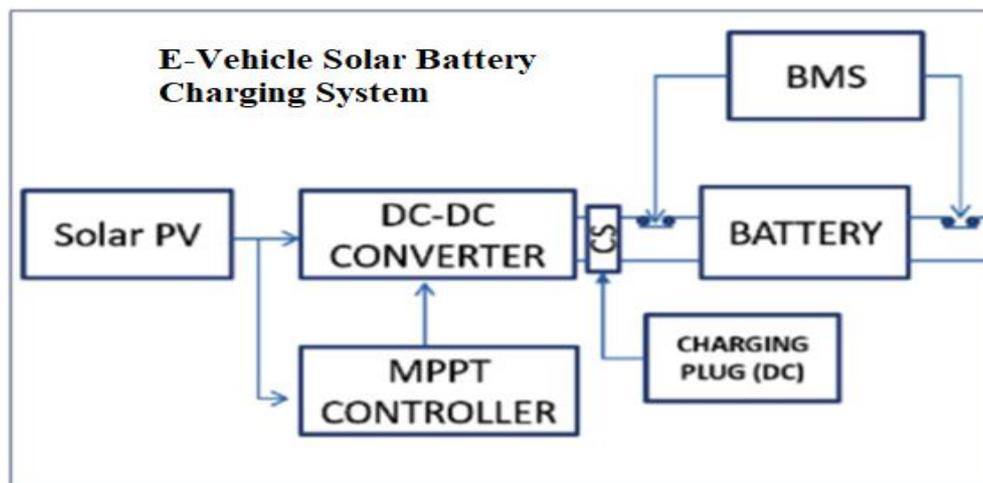
*Fig.1 E-Vehicle Solar Battery Charging System*
