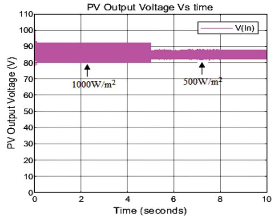
**Fig 4.3.2 PV output voltage vs. time at 1000W/m2 and at 500W/m2.**
