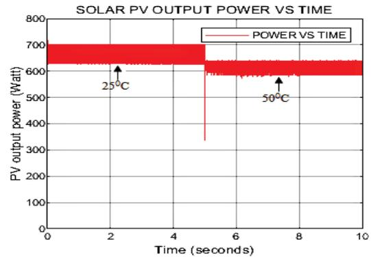
**Fig 4.3.4. PV output power vs. time at 25C and 50C and at 1000W/m2 and at 500W/m2.**
