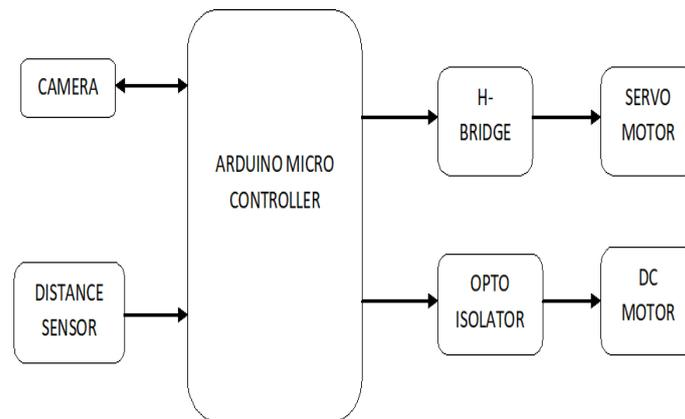
**Fig 2: Block diagram of Suggested system**
