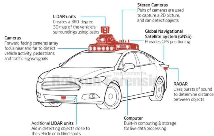
**Fig 3. Various sensors used in Autonomous car**
