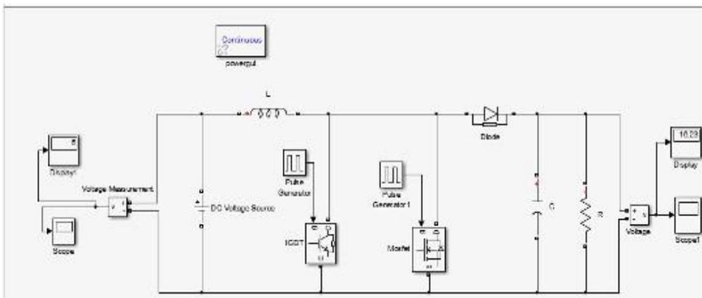
**Fig 5:** Boost converter simulink model
