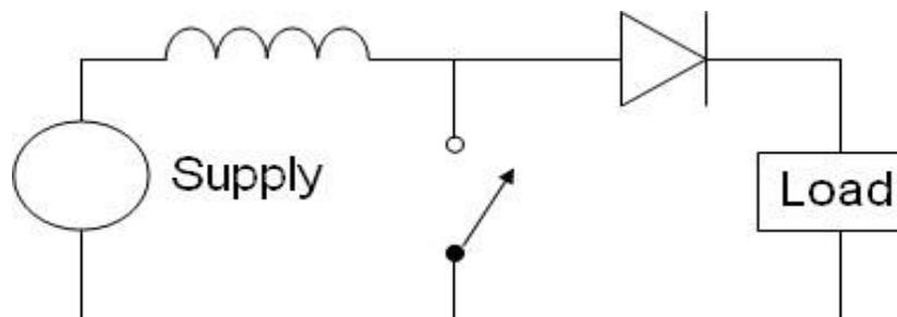
**Fig 1:** basic structure of boost converter
