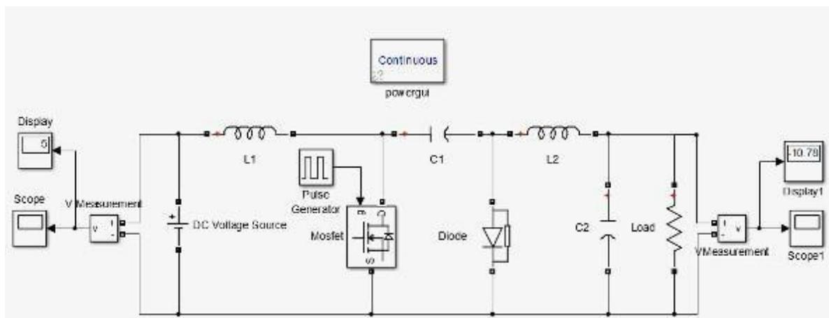
**Fig 8: Cuk converter Simulink model**
