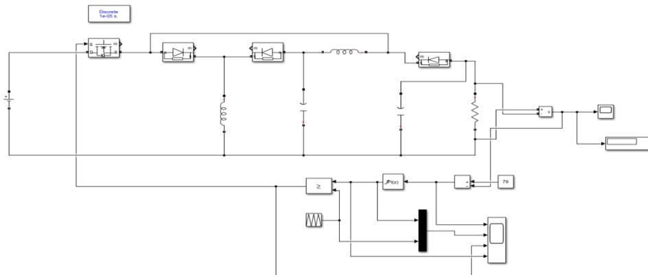
Fig.7.a.Simulation Model of PI Control of Ultra-lift Luo converter
