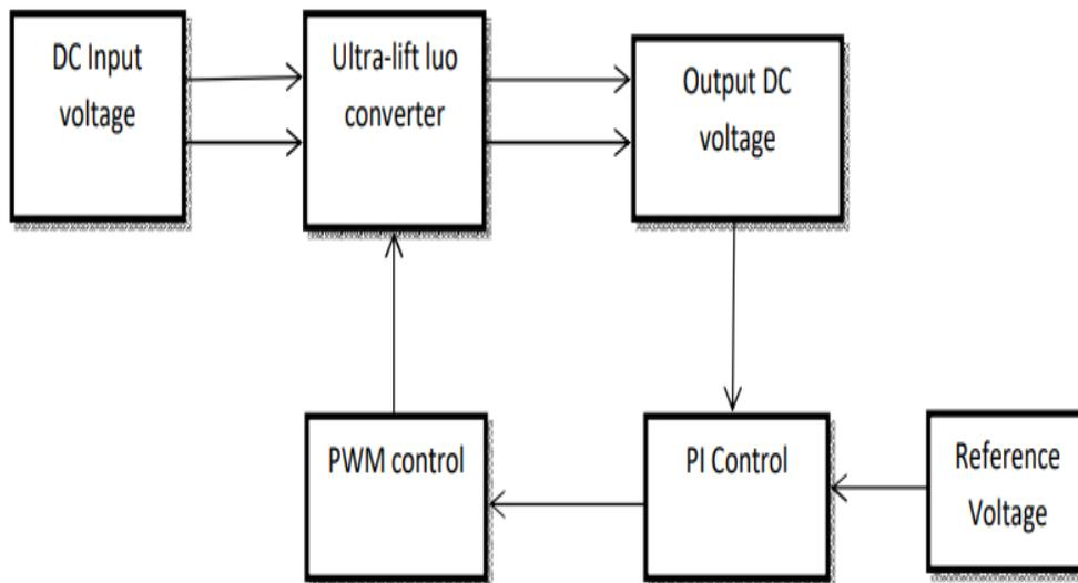
The DC input voltage is the power system voltage that uses only one polarity of voltage or current and have the constant, zero frequency which is applied to the Ultra-lift Luo converter. Ultra-lift Luo converter is a type of converter which boost up the voltage level by reducing the ripple content from the DC voltage.
