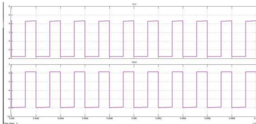
**Fig9:** Voltage across L2 and diode
