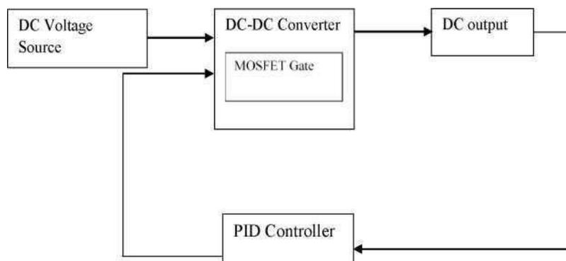
**Fig6:** Block diagram of converter using controller
