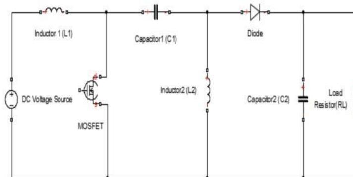
**Fig2:** Conventional SEPIC converter
