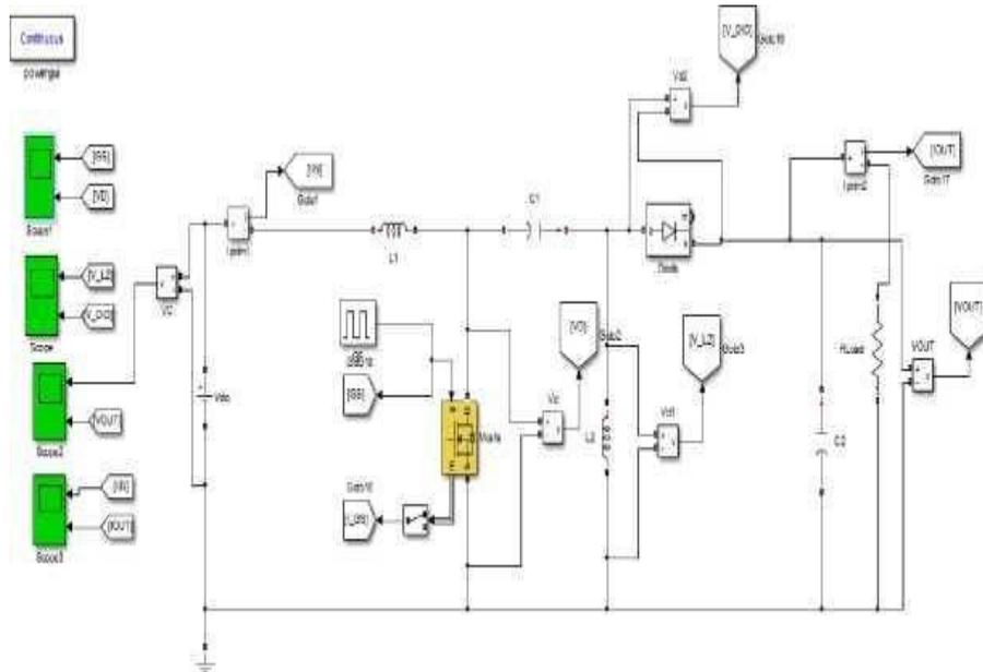
**Fig7:** Simulink diagram of convention SEPIC converter
