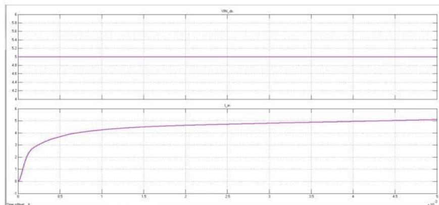
**Fig13:** Input voltage and input current of SEPIC using PID Controller
