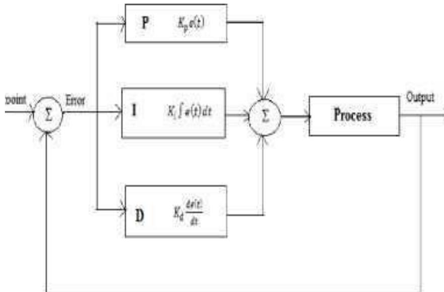
**Fig5:** PID Controller
