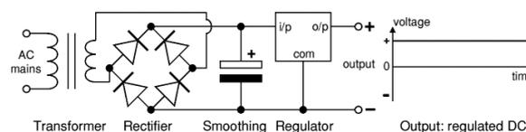
Figure 5.6 Transformer Rectifier Smoothing Regulator
