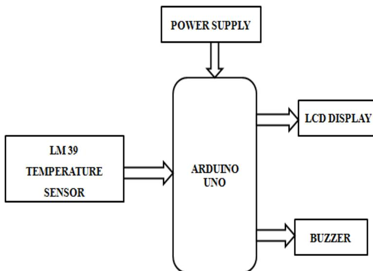
Figure 2.1 Block Diagram of Existing System
