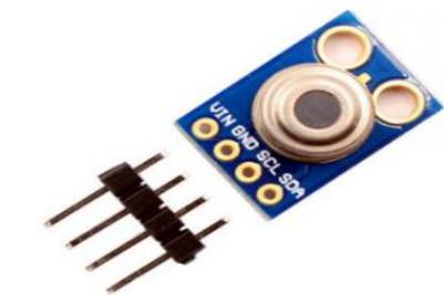
**Figure 5.9 MLX90614 Temperature Sensor**
