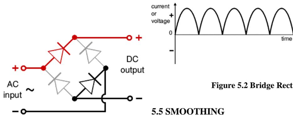
**Figure 5.2 Bridge Rectifier**
