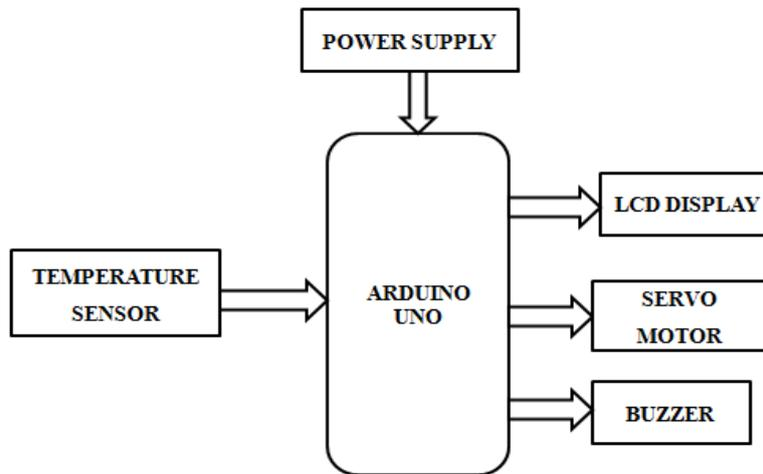
**Figure 3.1 Block Diagram of Proposed System**
