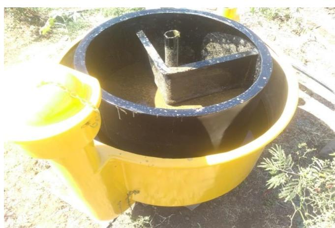
Fig6; Digester Inner side
