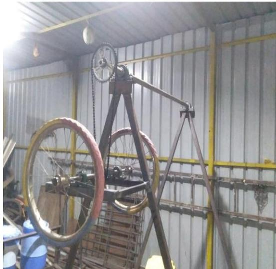
**Fig.8** Power generation using swing motion
