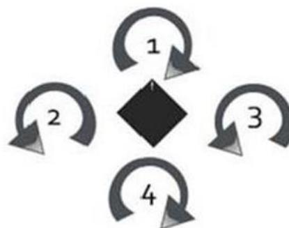
**Fig. 2 Initial rotation of wings**
