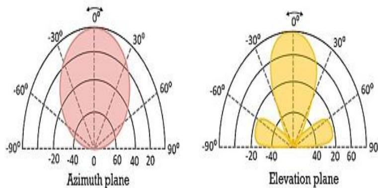
Fig 2: Radiation patterns of Microstrip Patch Antenna [16]
