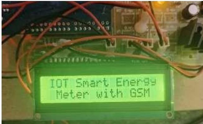
Fig3.4 Smart energy meter with GSM display 16*2
